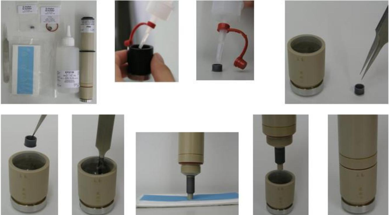
Air bubbles in the electrolyte can create pressure differences and generate a pumping effect that will dramatically increase the electrolyte use. It will also reduce the life time of the membrane as it will move with every pressure fluctuation.
